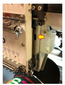
When oiling inside this hole, you are to hit the three points highlighted below:
