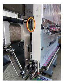
6. Needle Bars (springs behind take up levers)-1 drop on each needle bar spring weekly
