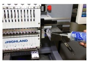
2. Behind head #2, oil in the two holes on the silver plate-2 drops in each hole daily
