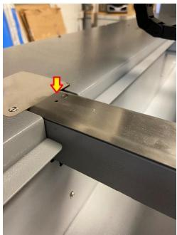
9. Thread Holding Device-Using the Alba-5 Lubricating Spray, spray the thread holding device from underneath it (roughly two or three sprays to cover all 15 needles) once per month
